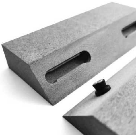
linear KV pocket - a simple straight milling
