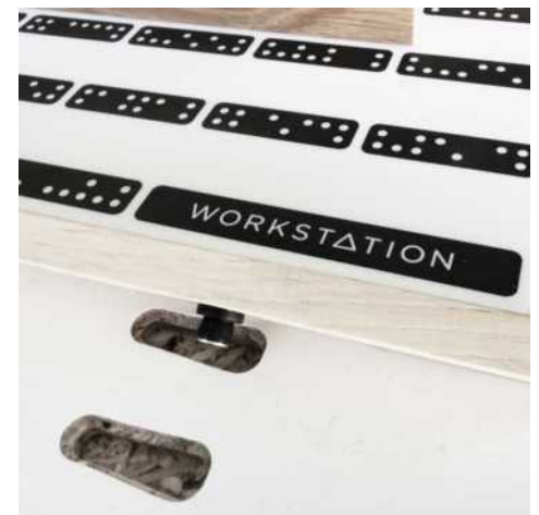
Free KV pocket milling for oak slats
